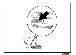
The Vehicle Identification Number (VIN) may be found in the location shown in the above illustrations. This number is used to register the vehicle. It is also used to assist your SUZUKI dealer when ordering parts or referring to special service information.
